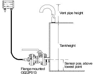
To ensure measuring accuracy a transducer type within the range no. 4, 5, 6, 7 and 8 is recommended.
